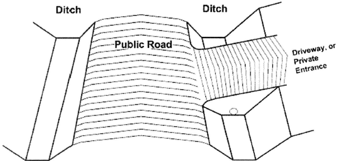
**Figure 8: Proper matching of driveway and road edge**
